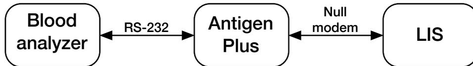
Other configurations are possible. On a computer with sufficient serial ports, it is possible to run Antigen Plus and the LIS on the same workstation. It is also possible to run Antigen Plus and the LIS on the same workstation using virtual serial port drivers. Please contact us if you have special needs.
